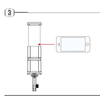
3. Place the phone/device in the middle of the bracket, be careful not to let the device fall.
