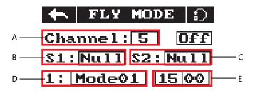
Different fly modes are assigned using combinations of switches. A 2-way switch will enable you to switch between modes 1 and 2,two 2-way switches will enable you to 4 fly modes, two 3-way switches will allow you to switch between all 9 fly modes. Use the table below to see which positions are assigned to each mode.
