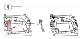
4. Place the spring hook assembly into position and hook the spring onto the hook located inside the transmitter.
