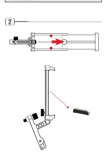
2. Move the slide to the highest position and remove the screws marked in red.
