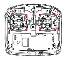
Take the transmitter apart, using a Philips screwdriver, remove the 8 screws marked in red.
