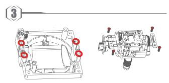
3. Loosen the assembly screws shown in fig.4 and remove the plate. Be careful to ensure no damage to cables.
