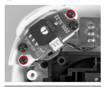
Take the transmitter apart, then use a screwdriver to remove the screws marked in red.
