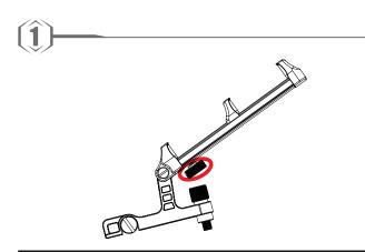
1. Loosen the locking screw by turning it anticlockwise.
