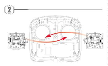
2. Swap the gimbals and rotate them 180 degrees, then line them up with the screw holes and replace the screws. (There is no need to disconnect the cables.)
