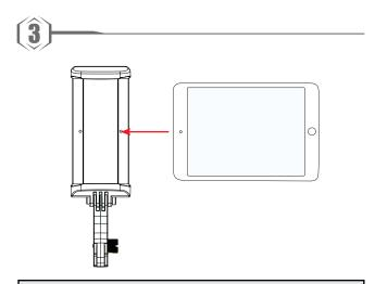
3. Move the your device into the centre of the bracket. Be careful not to let the device fall.
