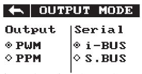
[PWM]: PWM output 1-6 channels outputting on the receivers 1-6 pins.
